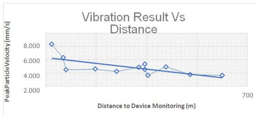
**Figure 2. Vibration Results In Non-Electric Detonators**
