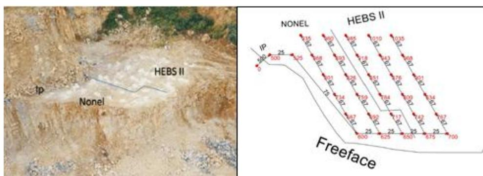
**Figure 3. Side by side explosion with the application of non-electronic detonators and delayers and HEBSII**
