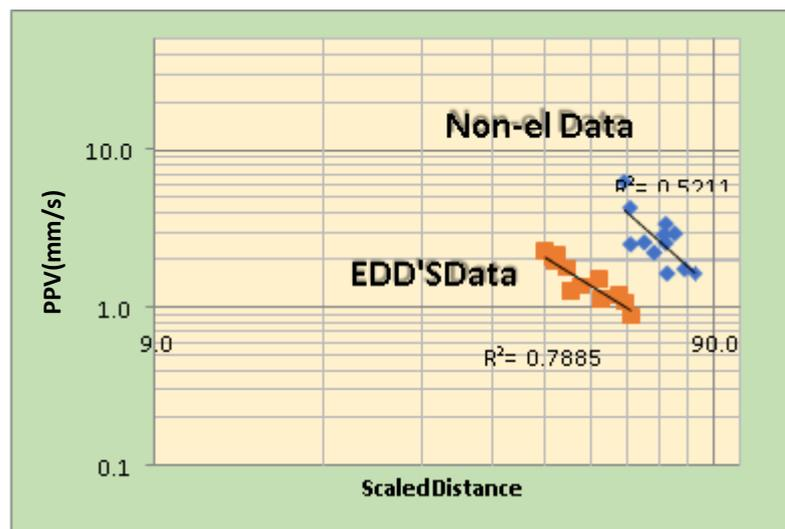
**Figure 6. Log Plot (PV versus Scale distance) comparing the results of electronic and non-electrical vibrations.**
