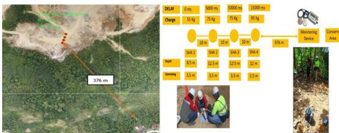
**Figure 1. Signature hole installation and point monitoring**
