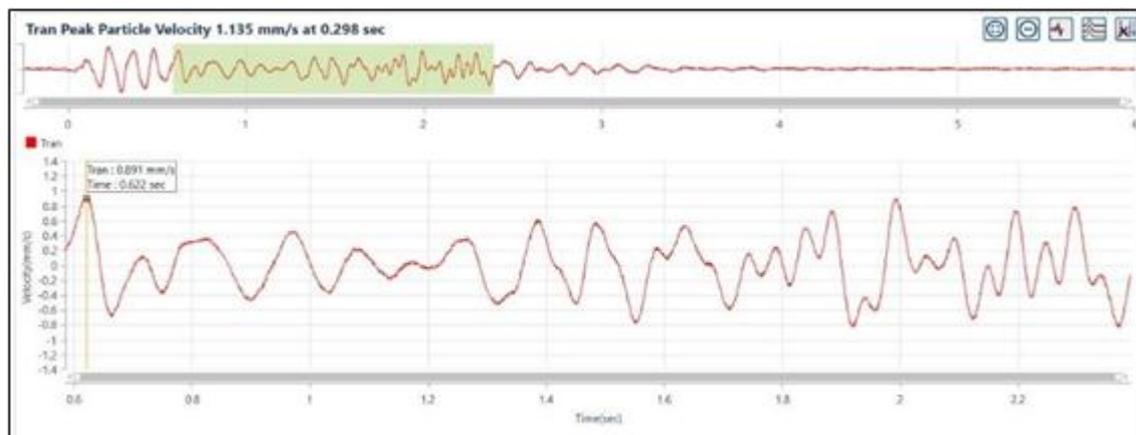
**Figure 5. Electronic Detonator wave analysis, peak vibration value 0.891mm/s**
