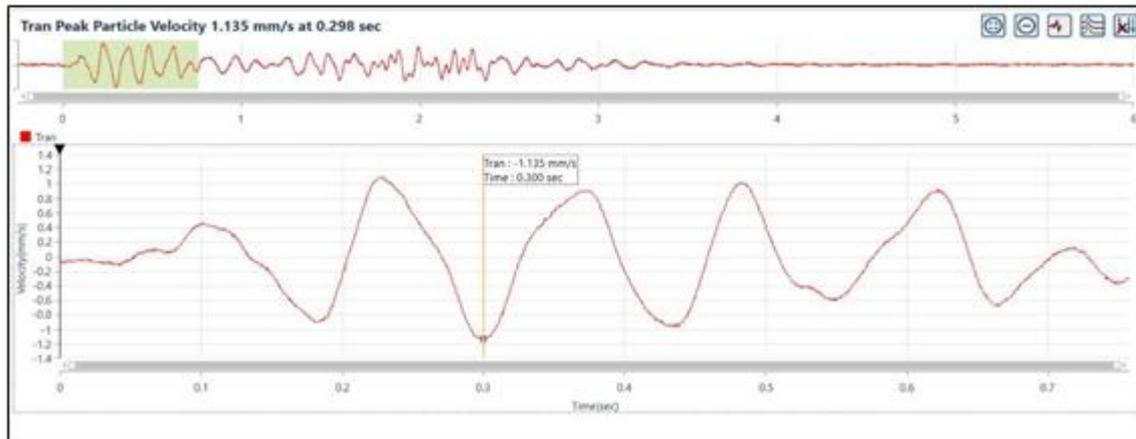
**Figure 4. Non-electric detonator wave analysis, peak vibration value 1.135mm/s.**
